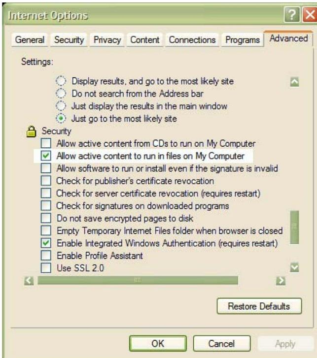
Figure 6. Check the security setting for active content on file on My Computer. See highlighted selection.
